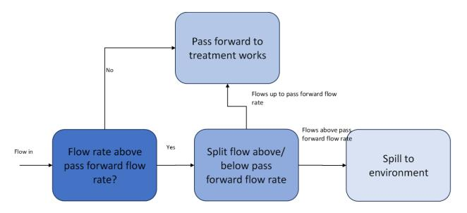
In this case at the 'split flow above/below pass forward flow rate' stage, flows were sent to spill to the environment before the pass forward flow rate was reached. This meant that more flow spilt to the environment than was permitted by the regulator.
